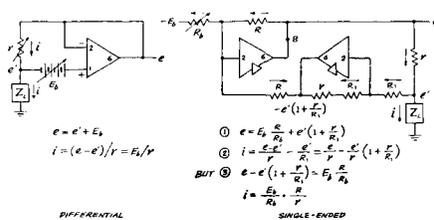
Fig. 1—Driving current to a grounded load.
