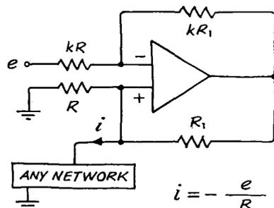
Fig. 2—Differential operational amplifier as current injector.
